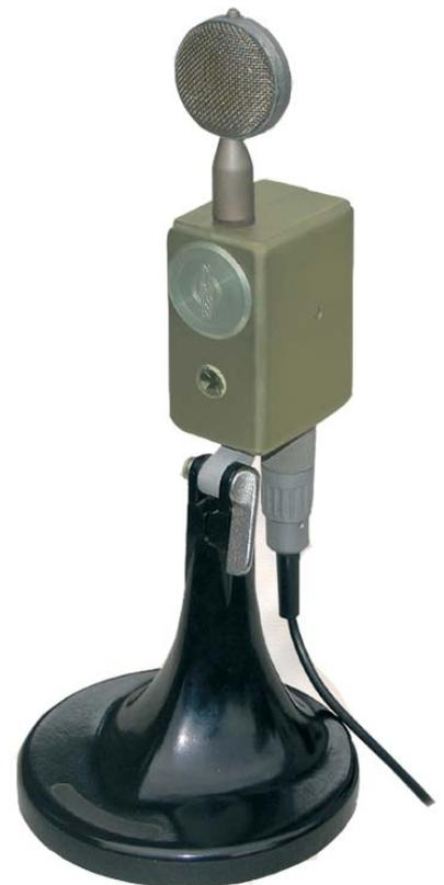
**1950** New condenser measurement microphones are developed and become part of the serial production.
